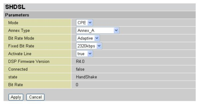
**Mode:** The SHDSL device can function as a CPE (Customer Premises Equipment) or CO (Central Office). Select CPE mode when the BiPAC 8500 is connecting to your ISP.
