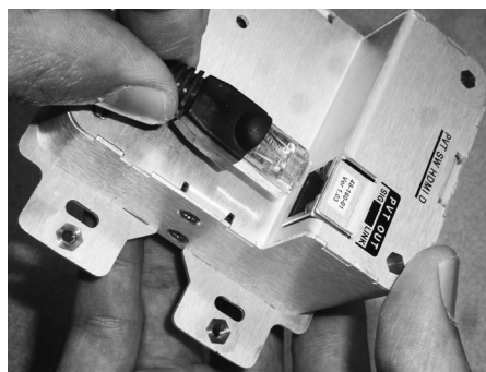
③a Connect the cables to the AV source input devices at each location.
