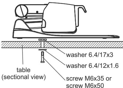
The Visualizer can also be fixed onto a table with the supplied table lock bolt in order to minimize the risk of theft.
