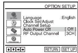
**3** Press  $\leftarrow/\rightarrow$  to change the setting. When changing the “RF Output Channel,” confirmation messages will appear. Press ENTER to confirm the messages.
