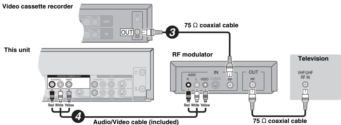
**d Connection with a television and cable box or DirecTV receiver (→ 17, C)**
