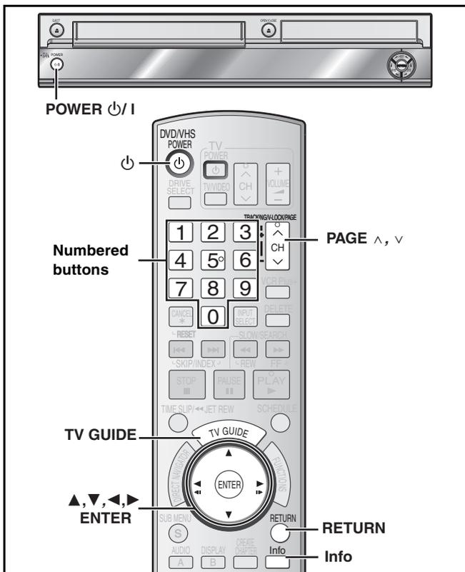
After plugging the unit into your household AC outlet and then pressing [⏻, DVD/VHS POWER] to turn the unit on for the first time, the unit starts language, TV aspect type and TV Guide On Screen® system setup.
