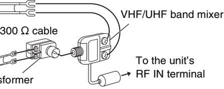
VHF/UHF band mixer<br>To the unit's RF IN terminal<br>300 to 75 Ω transformer    | VHF/UHF band separator<br>75 Ω coaxial cable<br>
