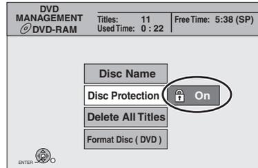
The lock symbol appears closed when the disc is write-protected.
