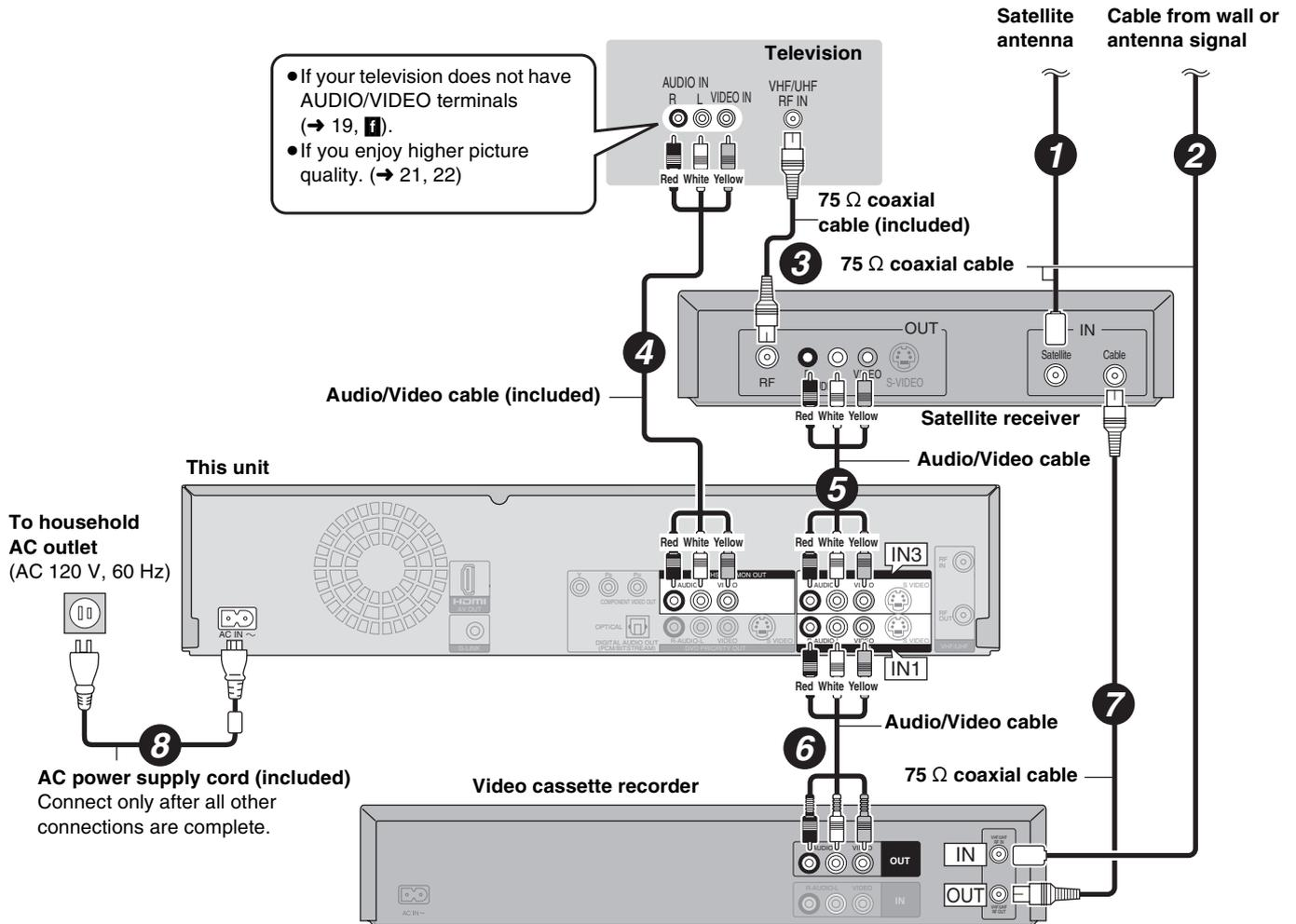
**If your television does not have AUDIO/VIDEO terminals, an RF modulator is necessary**
