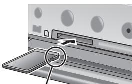
Insert the card label up with the cut-off corner on the right.
